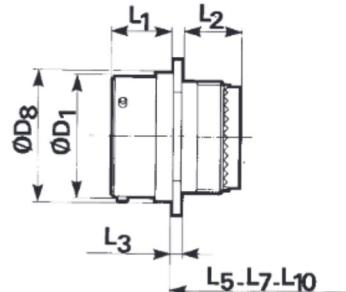
cable connecting receptacle backshell assembly overall length
