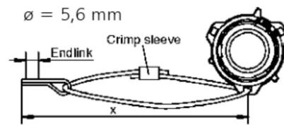
**Adaptor for Flex Tube****For 2-way Plug and Receptacle**
