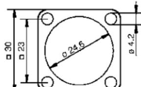
**Adaptor for Flex Tube****For 1-way Plug and Receptacle**
