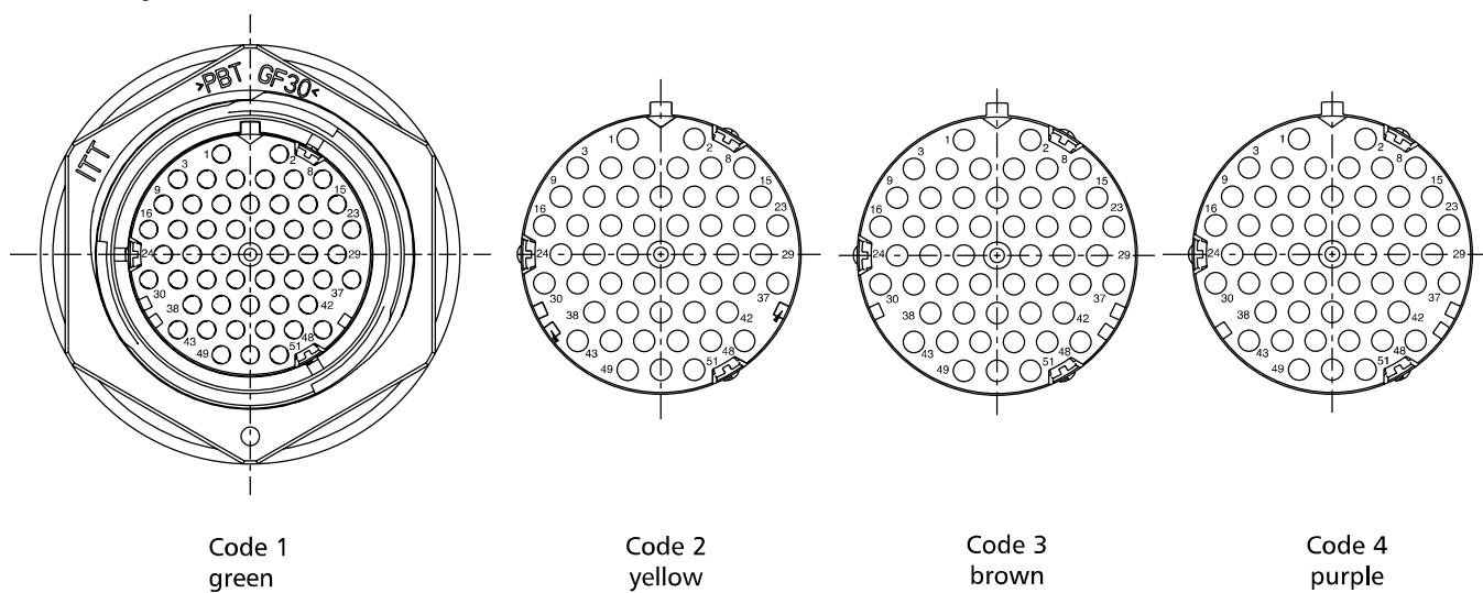
Note: The connectors offer both mechanical keying and visual coding by different colors.
