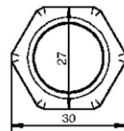
**Flange Gasket****For Flange Receptacle, High Power 1-way**
