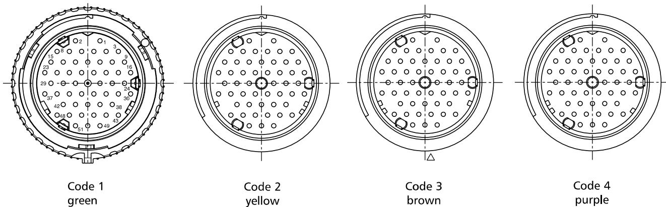
Note: The connectors offer both mechanical keying and visual coding by different colors.
