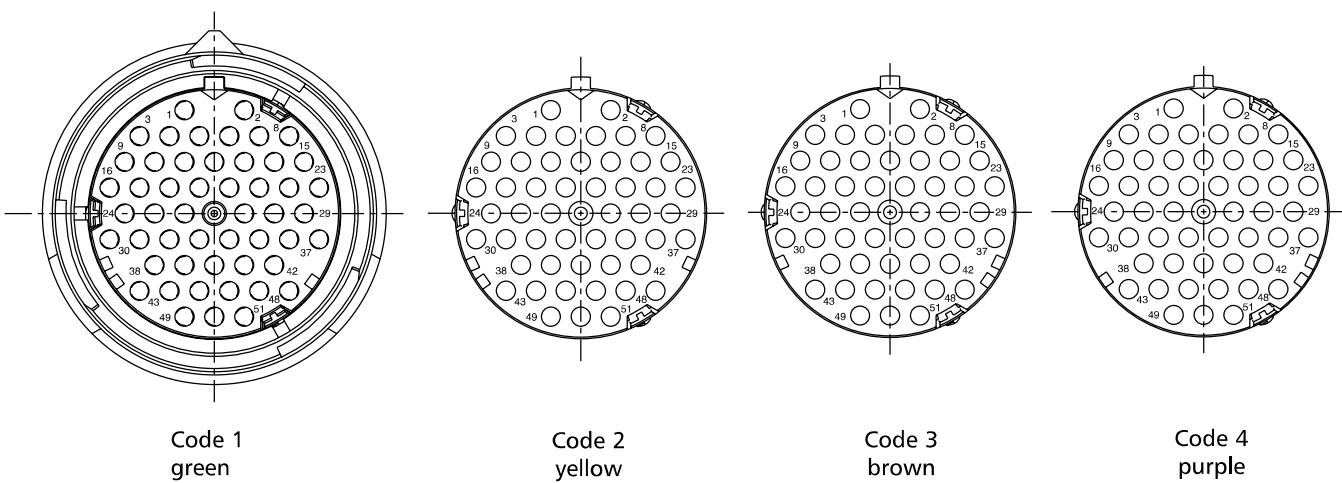
Note: The connectors offer both mechanical keying and visual coding by different colors.
