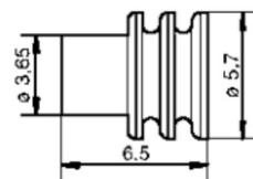
**Flange Gasket****For Flange Receptacle, 4-way**
