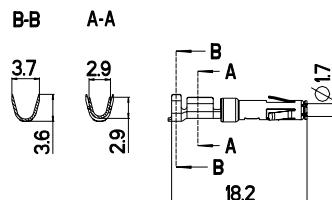
**Pin Crimp-Contacts 1,6 mm Standard Tinned, 3000 contacts per reel**
