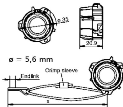
**Cable Seal for Cable (in acc. to DIN 670722 FLY/ DIN 72551 FLRY) High Power 1-way**
