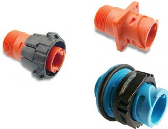
The APD 1 / 2-way connectors are derived from ISO 15170 and adapted to applications requiring high power. These versions cover wire ranges from 16 mm<sup>2</sup> up to 50 mm<sup>2</sup> power and a power consumption up to 245A. The combination of small size and high power make them an ideal solution for many applications.
