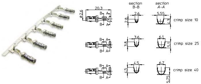
**Pin Crimp-Contacts Standard Tinned, 3000 contacts per reel**
