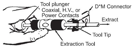
The CET-CGB-2 tool extracts all coaxial, high power and high voltage contacts (plug and receptacle).
