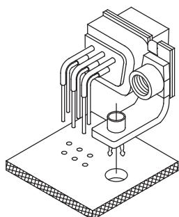
**Alternate 50 Ohm Coaxial Configuration**
