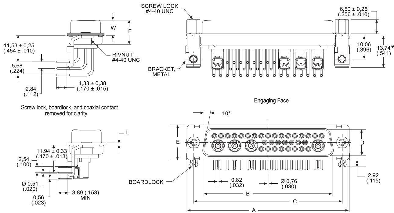
Screw lock, boardlock, and signal contacts removed for clarity
