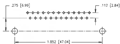
PCB layout for .590 footprint with Modifier Options B or D only
