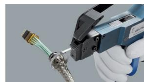
**STEP 3:** Use the tool part number 057-0450-00 to tighten the ring around the shielded braid over the chimney.
