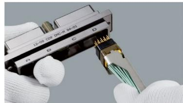
**STEP 4:** Slide the tool around the cable. Then push the tool inside the housing until butting.
