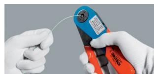
**STEP 5:** Tighten the crimping tool.
