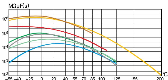
Fig. 4 : Insulation resistance change versus temperature
