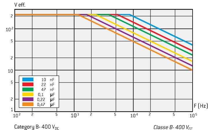
The rated voltage values given comply with Class B specifications of the NF C 83153 standard.
