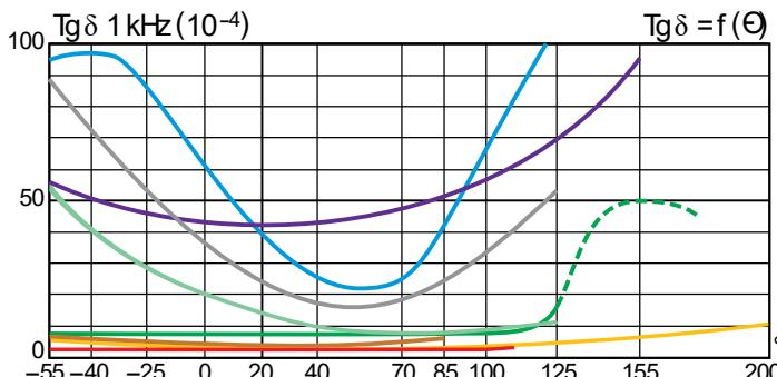
Fig. 3 : Loss angle change versus temperature
