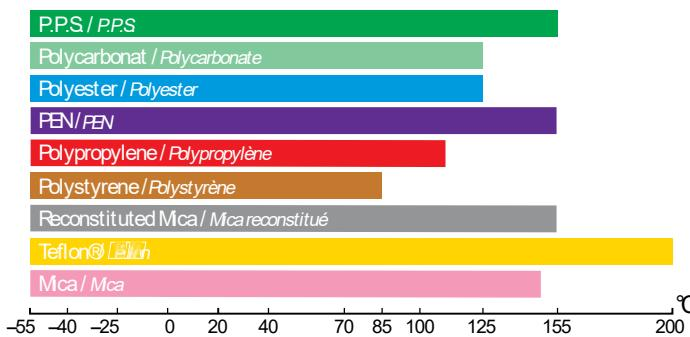
Fig. 1 : Ranges of operating temperatures
