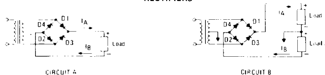
FIGURE 12 – BASIC CIRCUIT USES FOR BRIDGE RECTIFIERS
