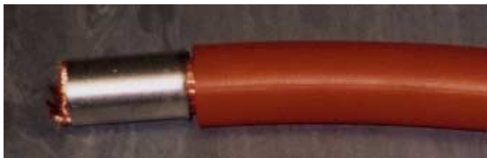
Figure 11. Showing Reduction Sleeve Fitted
