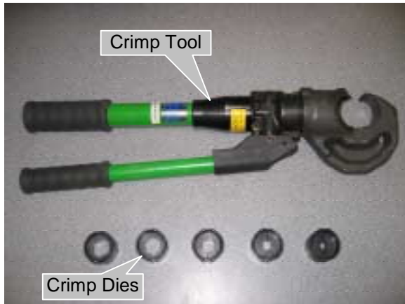
Figure 4. Example Of A Typical Hydraulic Crimp Tool With Dies
