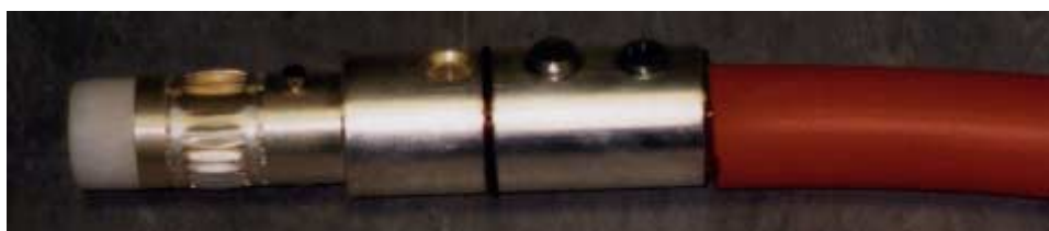
Figure 12. Showing Contact With Set Screws Fitted Over Cable And Reduction Sleeves
