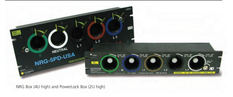
To simplify PowerLock connections to a fixed unit, five port boxes are available with built in safety features. Each box offers a sequential mating feature that requires the individual lines be connected in order, Ground first then Neutral followed by the three Phases and disconnected in the reverse order. Once connected the boxes can be locked to prevent unauthorized disconnection.
