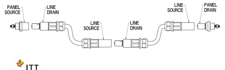
PowerLock connectors feature a bayonet coupling mechanism with a secondary locking pin. When a pair of connectors are mated and fully turned to engage the bayonet, the spring loaded secondary locking pin on the Drain connectors, snaps into a slot on the Source connector; a special release key is then required to uncouple the connectors.
