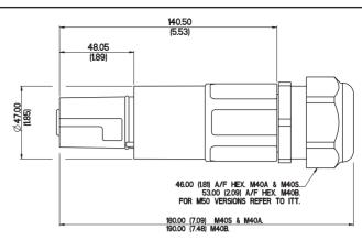
Line Drain is the connector with a female contact which is not normally the live part, however they are fitted with a spring loaded plastic cap that prevents accidental finger touching of the contact, and the connector meets IP2X requirements. Contacts are available to suit cable conductors from 25mm<sup>2</sup> to 300mm<sup>2</sup>.
