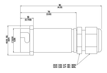
Female Panel Socket with cable fixing
