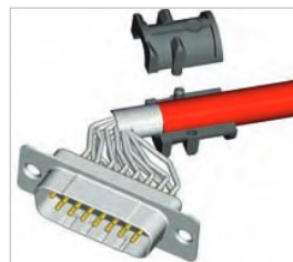
Attach the strain relief around the cable
