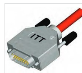
Assemble the other half (screwing force: 100-120 Ncm)
