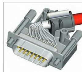
Mount connector and cable into the backshell
